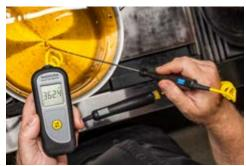
connect to your host device (iOS or Android) via the app, probe the item to be measured, and press the button to securely transmit your temperature data up to 150 feet.
